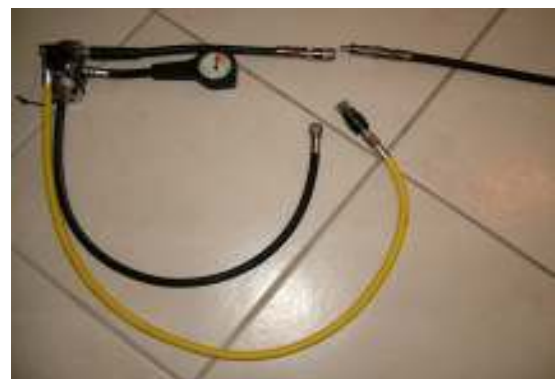
Stage Tank 1st Stage and hoses. Yellow hose to second stage reg. Black hose with DIN connector for drysuit inflation, MGBP operation or DSMB inflation etc
