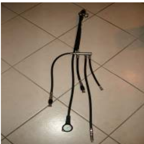
Hoses, FFM second stage inlet hose on left. SPG. ADV supply. Manifold inlet hose from stage tank. Wing inflator hose
