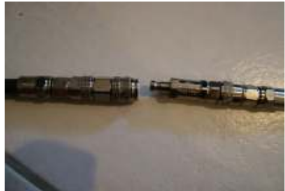
M&J Quick Disconnect and Check Valve direction of flow is L to R toward the manifold
